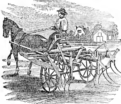
PATENT HAY TEDDER, Or Machine for Spreading and Turning Hay.
